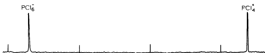
FIG. 7. ^{31}\text{P} NMR spectrum of polycrystalline phosphorus pentachloride with magic angle spinning. The two lines arise from the differently shielded \text{PCl}_4^+ and \text{PCl}_6^- ions of which the solid is composed. Markers at 1 kHz intervals (Andrew et al. , 1960a,b, 1966).
